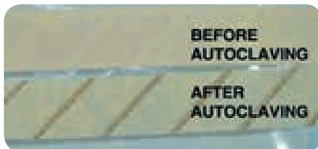
Use to seal bags and boxes. Integral marking changes colour when passed through a full cycle. Note that a change in colour of the tape does not necessarily guarantee that the contents of the bag or pack are sterile.
