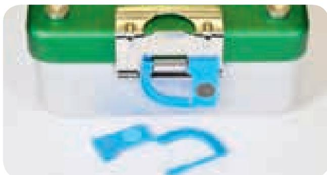
Anti-tamper Security Padlock with steam sterilisation indicator spot. Spot colour changes from pale blue to brown. Single use only. Padlock has to be broken to be removed.
